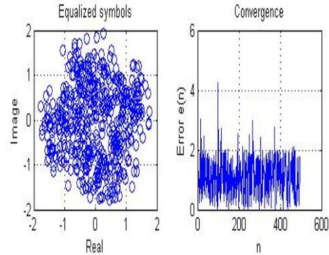
Figure 2.3 Symbol equalization Figure 2.4 MSE Convergence when Maximum sample size is 500 and SNR = 15Db
